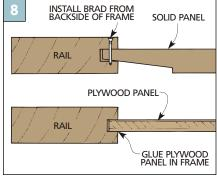
**Securing Panel.** A solid panel floats in the frame. Use a brad to keep it centered. A plywood panel can be glued in.
