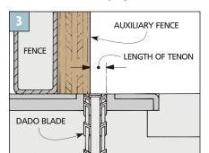
To use a dado blade, first bury it in an auxiliary fence (*Fig. 3*). Then adjust the fence to set the length of the tenon.
