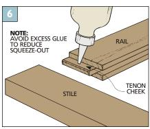
**Gluing Up.** A thin bead of glue spread evenly on each cheek of the tenon is all that's needed when gluing up the joint.
