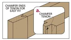
**Chamfer Tenon.** Small chamfers on the ends make it easier to fit a tenon into a groove during assembly. It also provides some space for excess glue.
